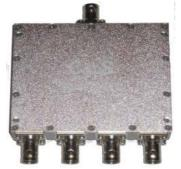
The SP-4-2-75-5 is a high performance combiner splitter designed for satellite IF signals. The case is machined from Aluminium alloy and has a Nickel plated finish. It is fitted with high performance 75 ohm BNC connectors..
